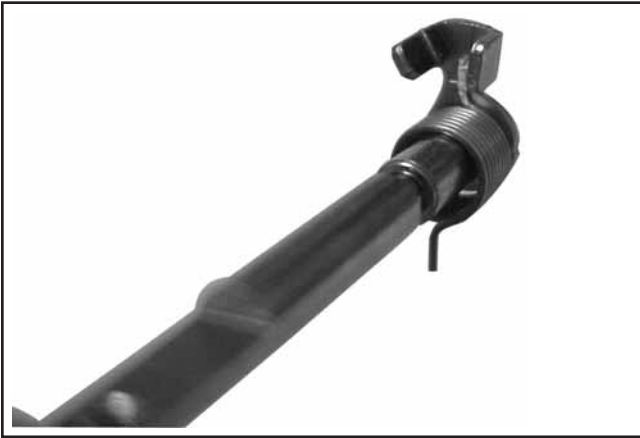
Figure 5-31. Choke Shaft and Spring Details.
