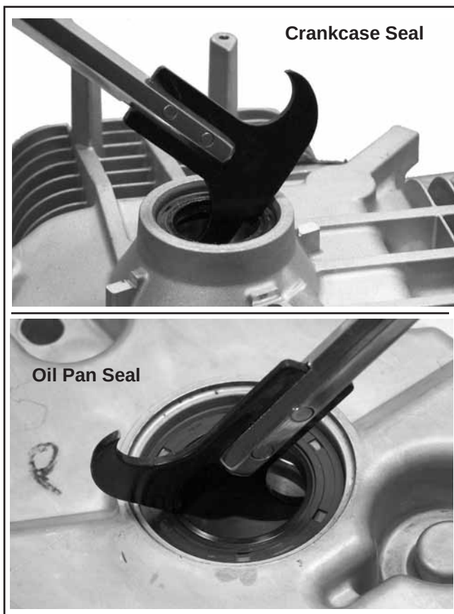
Figure 8-53. Removing Oil Seals.
