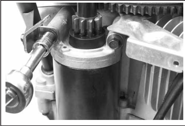
Figure 10-79. Installing Starter, Lift Bracket, and Oil Fill/Dipstick Tube.
