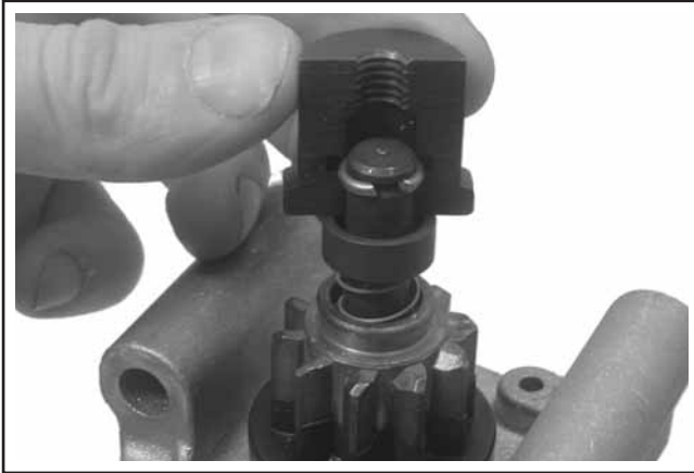
Figure 7-31. Assembling Inner Half of Removal Tool Around Armature Shaft and Retaining Ring.
