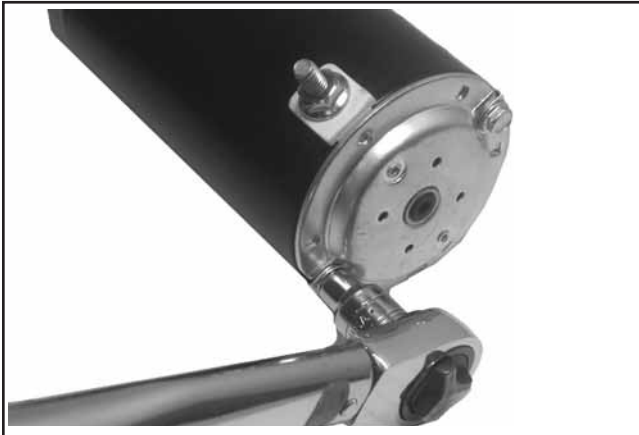
Figure 7-37. Installing and Torquing Thru Bolts.
