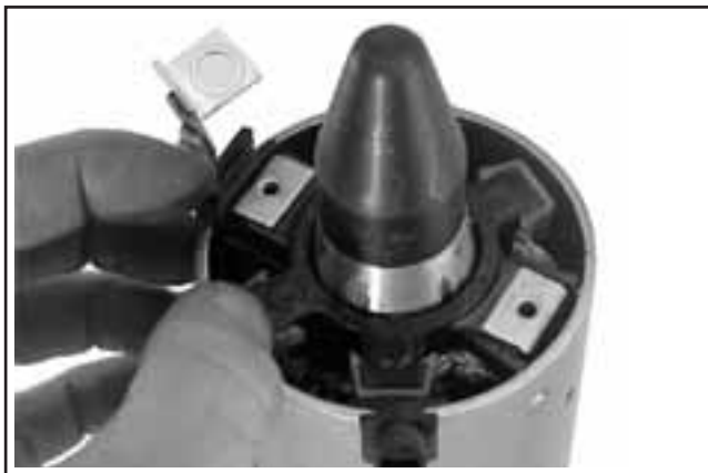
Figure 7-64. Installing Brush Holder Assembly using Tool with Extension.
