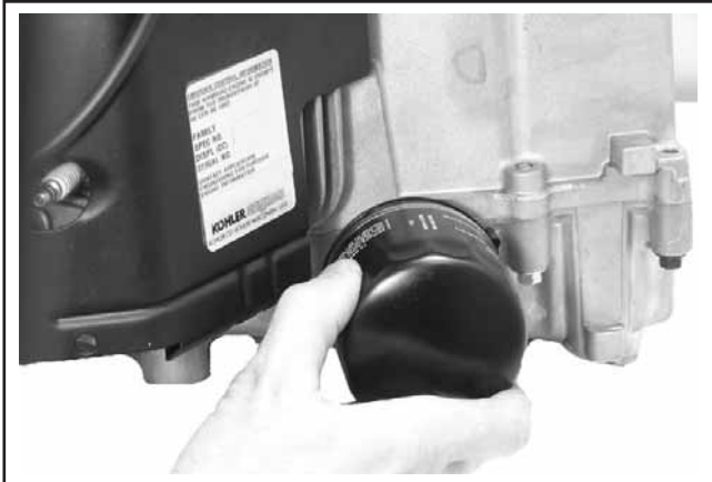
Figure 10-84. Installing New Oil Filter.
