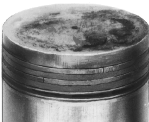
Stuck, Broken Rings
