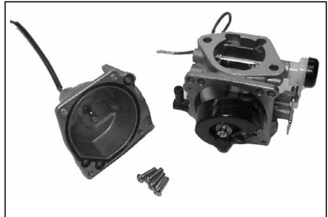
Figure 5-9. Fuel Bowl Removed from Carburetor.
