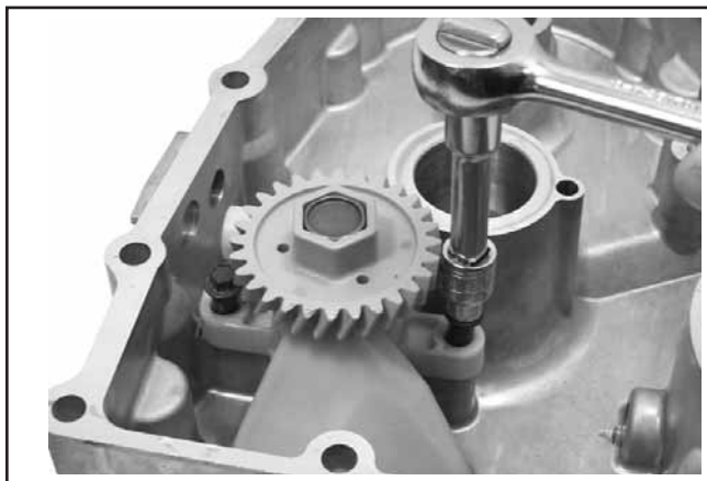
Figure 9-15. Removing Oil Pump Mounting Screws.
