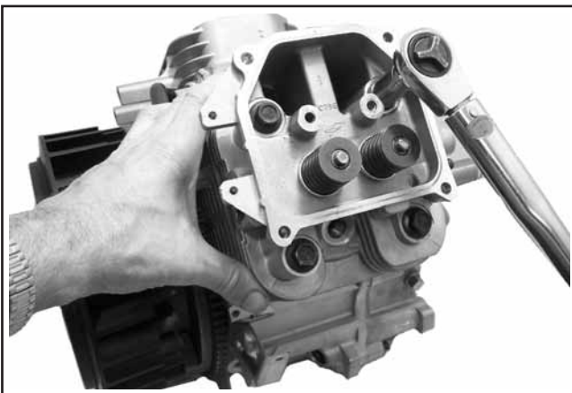
Figure 10-45. Torquing Cylinder Head Fasteners.
