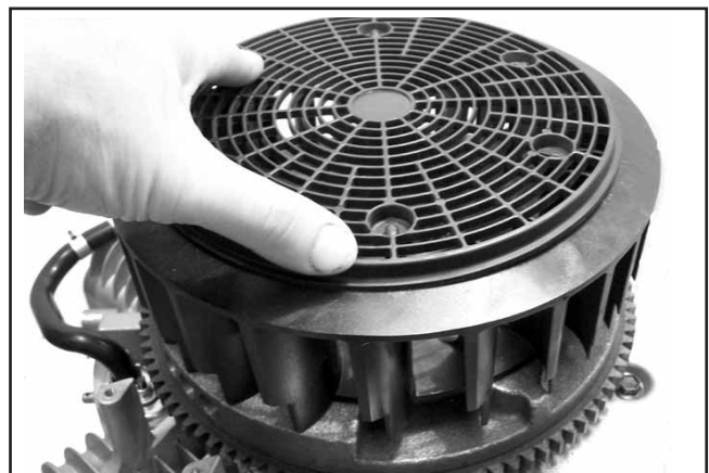
Figure 10-39. Installing Grass Screen.
