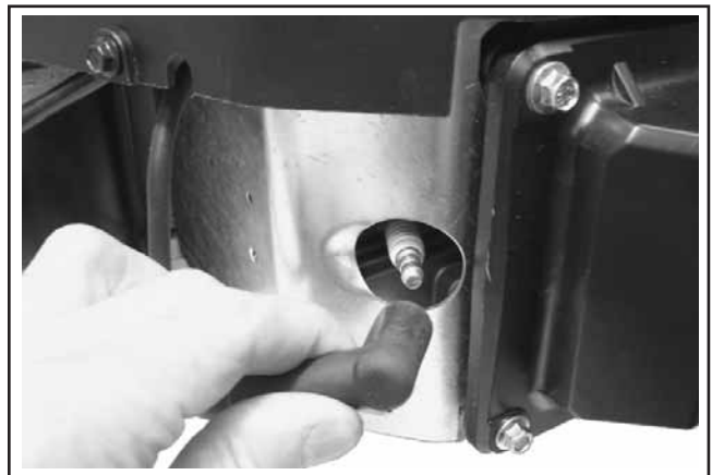
Figure 8-1. Disconnect Spark Plug Leads.
