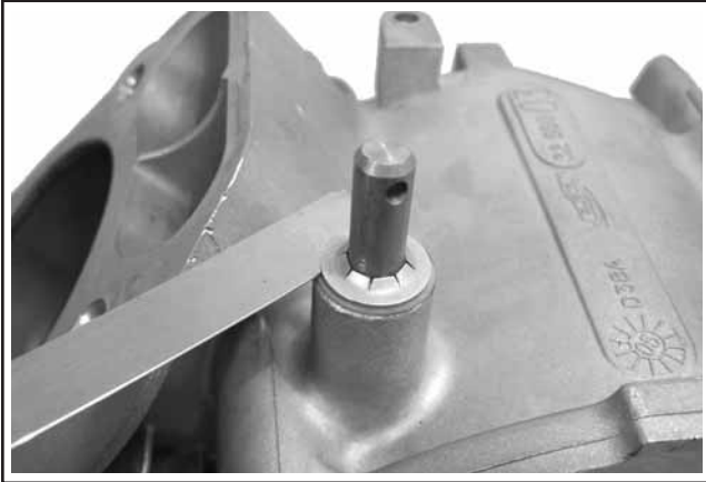
Figure 10-6. Setting Governor Shaft Endplay.
