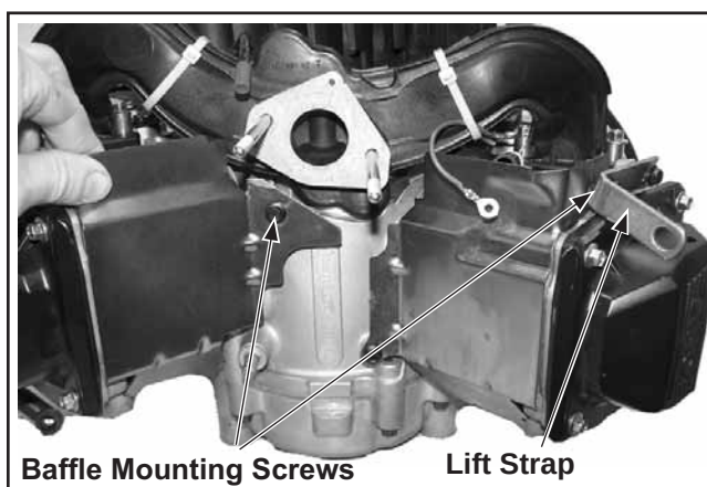
Figure 10-64. Installing Inner Baffles and Lift Strap.
