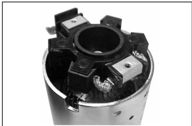
Figure 7-61. Installing Brush Holder Assembly with Supplied Tube.
