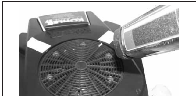
Figure 7-12. Check For Timing Advance.
