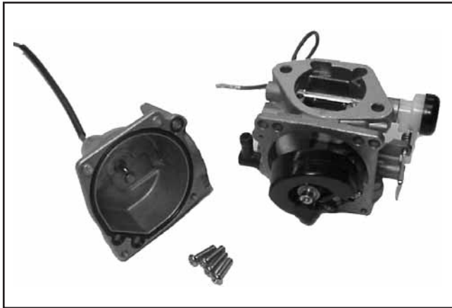
Figure 5-15. Fuel Bowl Removed from Carburetor.
