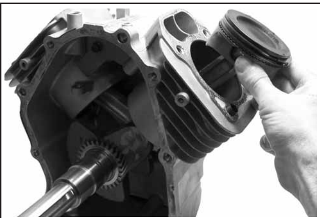
Figure 8-50. Removing Connecting Rod and Piston Assembly.
