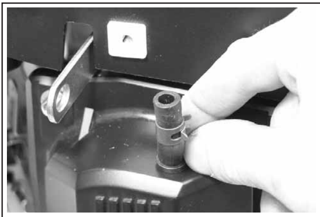
Figure 10-81. Installing Pulse Hose.
