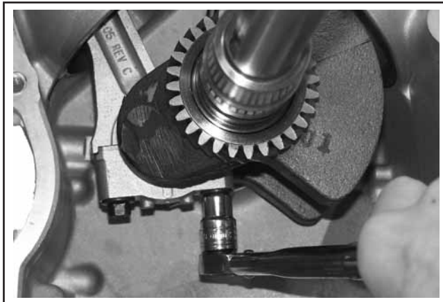
Figure 10-11. Torquing Connecting Rod End Cap.
