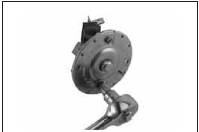
Figure 7-53. Removing Brush Holder.
