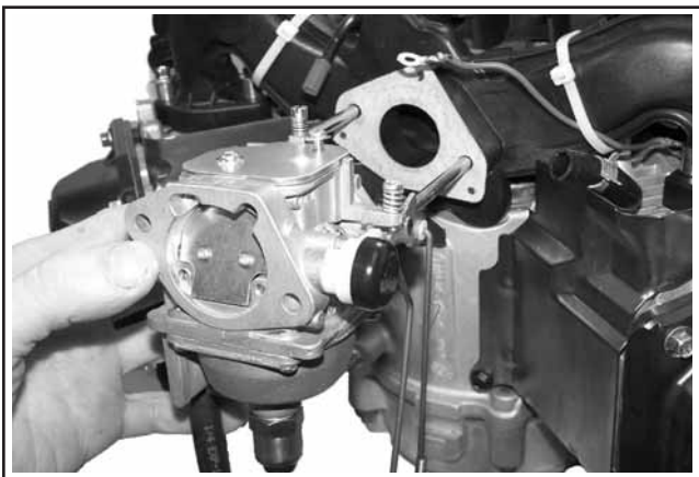
Figure 10-66. Installing Carburetor, Throttle Linkage and Governor Lever.
