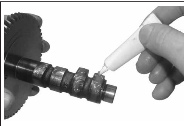
Figure 10-14. Apply Camshaft Lubricant to Cam Lobes.
