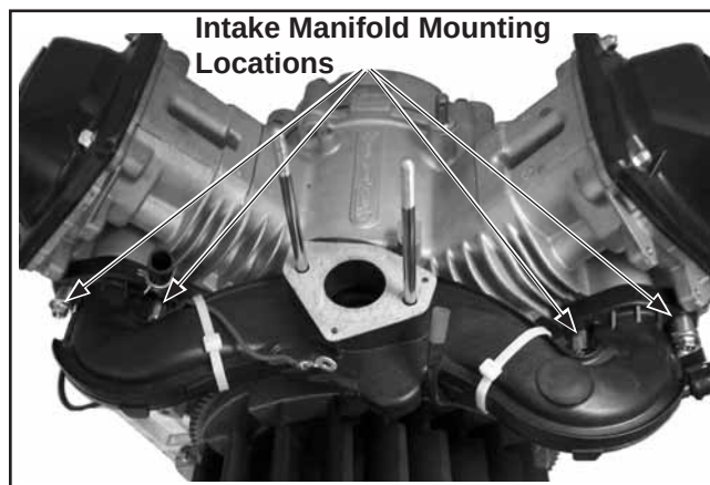
Figure 8-22. Intake Manifold Mounting Locations.
