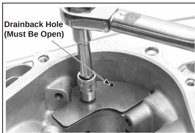
Figure 10-4. Torquing Breather Cover Screw.
