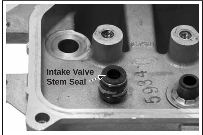
Figure 8-34. Intake Valve Stem Seal* (Some Models).
