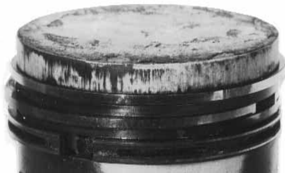
Overheated or Deteriorated Oil
