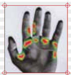
Without soft-grip coating: extreme pressure points
